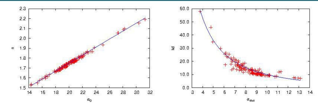
$n = (0.0403 \pm 0.0082)\alpha_0 + (0.9438 \pm 0.1650),$   $kd = \frac{(558.1472 \pm 5.5233)}{\alpha_{\min}^{(1.67 \pm 0.01)}} - (1.9188 \pm 0.1926),$  $\alpha_{\min} \text{ provides information about the texture of the surface of the surfa$
