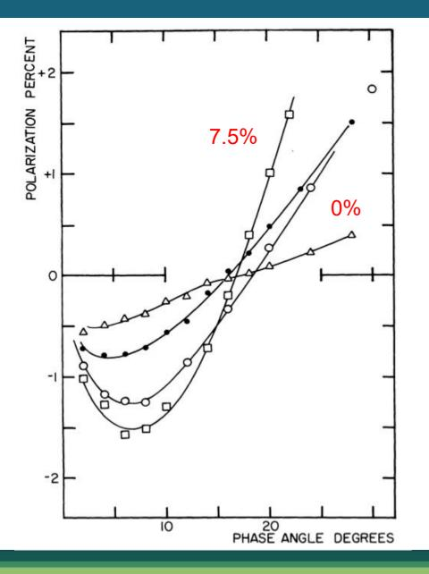
Polarimetric curves of silicates mixed with different amount of carbon
