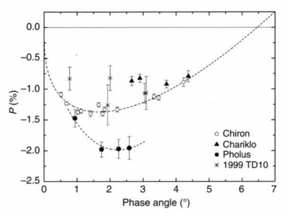
Polarization curve has a deep negative value at small phase angles.
