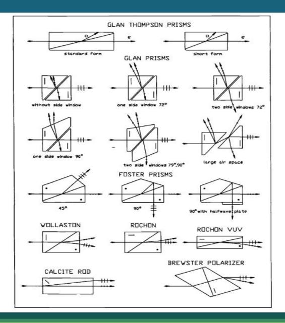
Some polarizers used in different instruments
